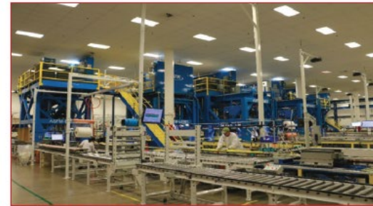
Automated stiffener forming (ASF) for linear stringers
